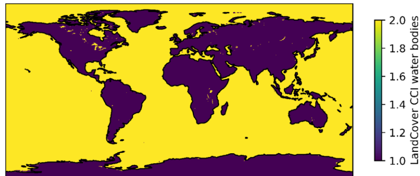
Figure 4-2: Mask of water bodies (oceans and inland open water surfaces) as resampled from 150 m-resolution map provided by the LandCover CCI, © ESA Climate Change Initiative - Land Cover led by UCLouvain (2017).
